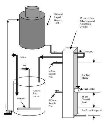
Figure 1. Schematic of peat adsorption and absorption system
